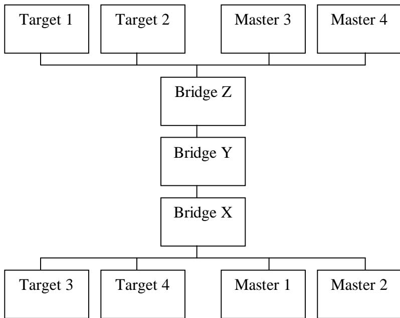
**Figure 26. Example PCI System**
