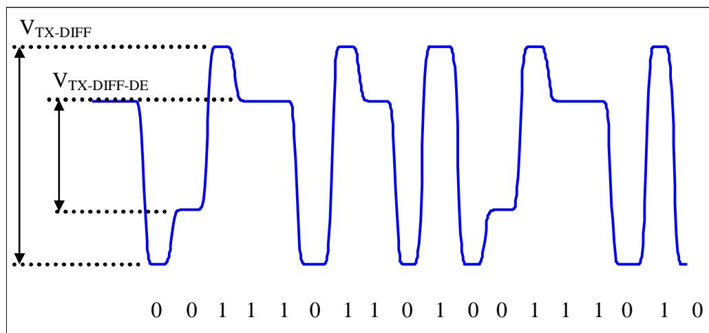
**Figure 51. Differential transmitter post-cursor de-emphasized waveform**
