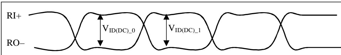
**Figure 35.  $V_{ID(DC)}$**
