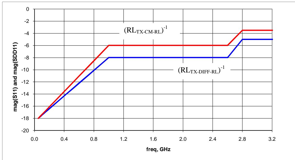
**Figure 50. Transmit return loss mask**
