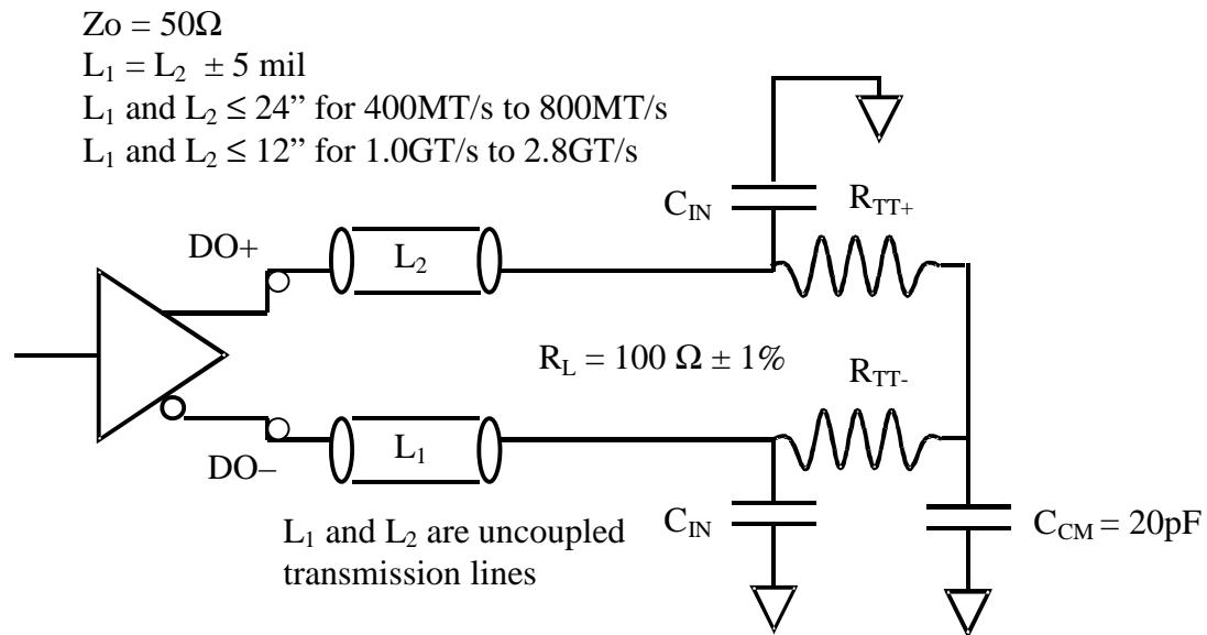
**Figure 37. AC Reference System Load** (See Table 168 for  $C_{IN}$ ,  $R_{TT+}$  and  $R_{TT-}$ )
