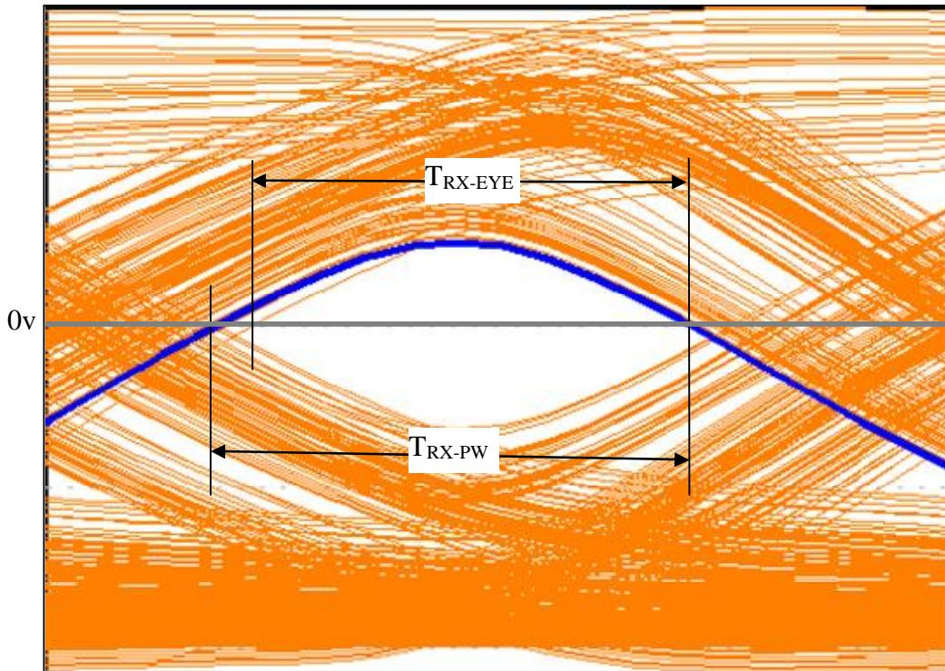
**Figure 60. Receiver cumulative eye showing min-pulse width**
