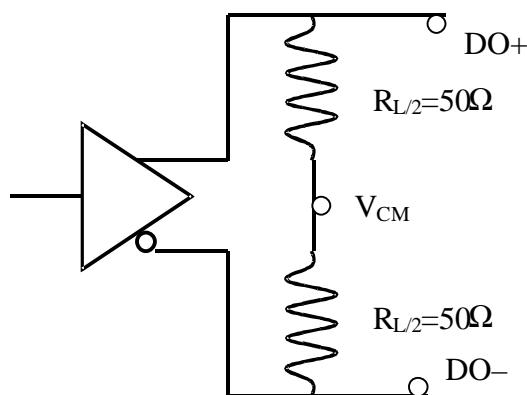
**Figure 31. DC Output Reference System Load**
