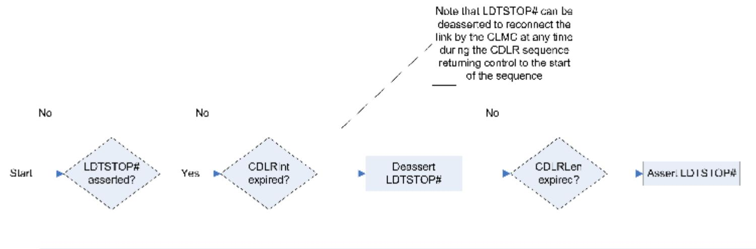
**Figure 13. CLMC Sequencing Diagram for CDLR**
