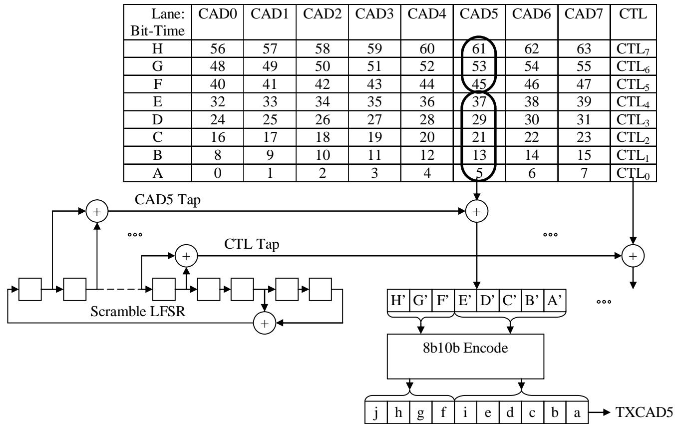
**Figure 4. Gen3 Transmitter Order of Operations**
