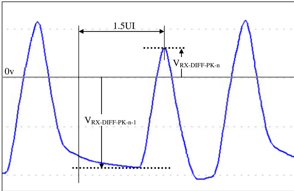
**Figure 61. Receiver adjacent bit ratio**
