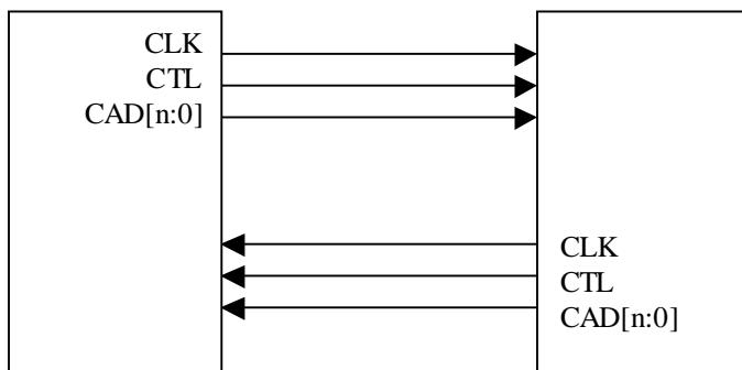
**Figure 1. HyperTransport<sup>TM</sup> I/O Link**
