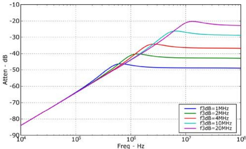
**Figure 49. System reference clock jitter rejection**
