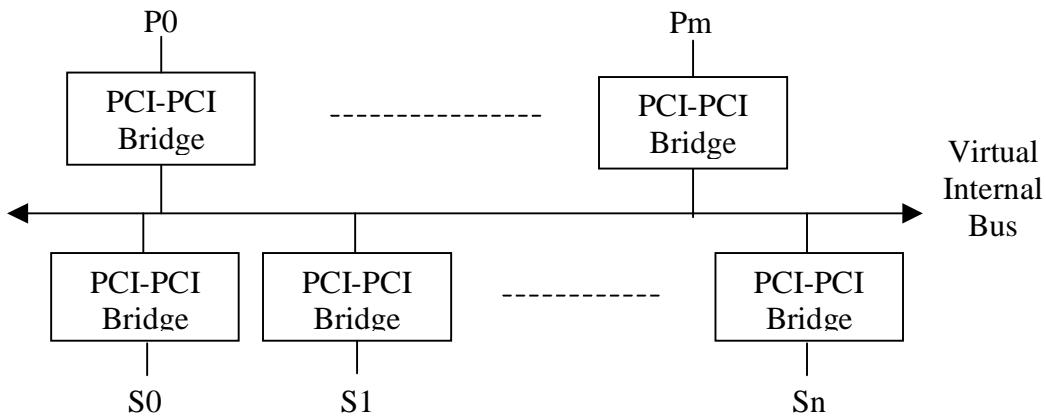
**Figure 29. Logical Model of a Switch**
