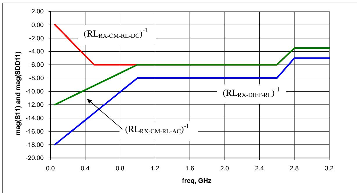
**Figure 58. Receiver return loss mask**
