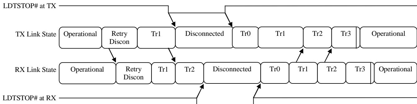
**Figure 20. Example LDTSTOP Disconnect Sequences**
