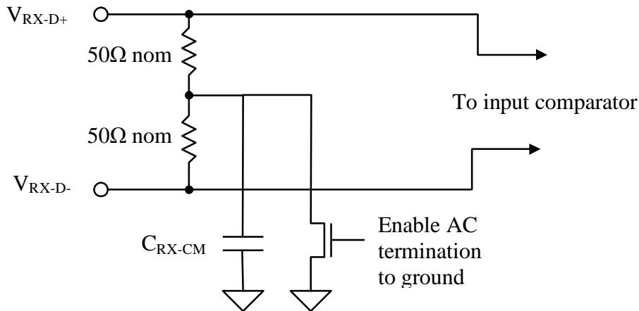
**Figure 59. Receiver input termination**
