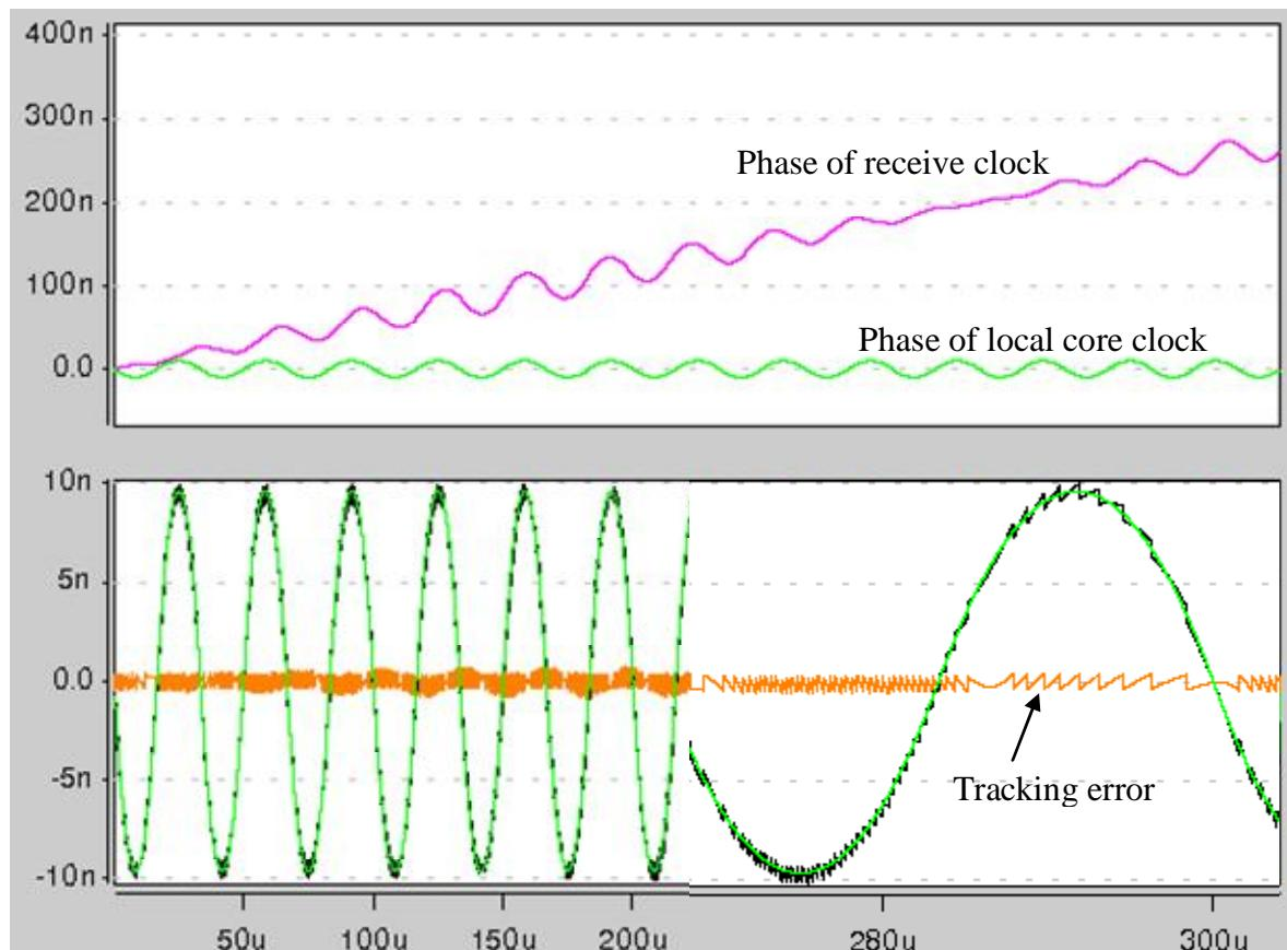
**Figure 65. Phase tracking across receiver sync-fifo**
