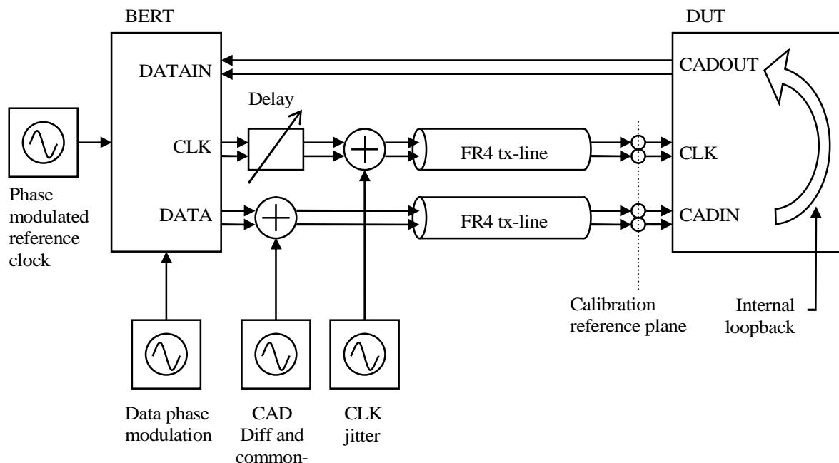
**Figure 63. Receiver input compliance test setup**
