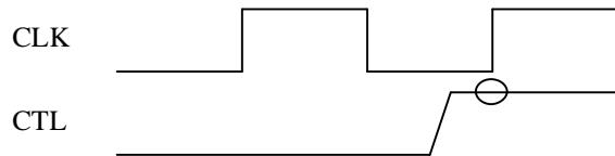
**Figure 16. Sync Sequence Timing for Link Initialization**
