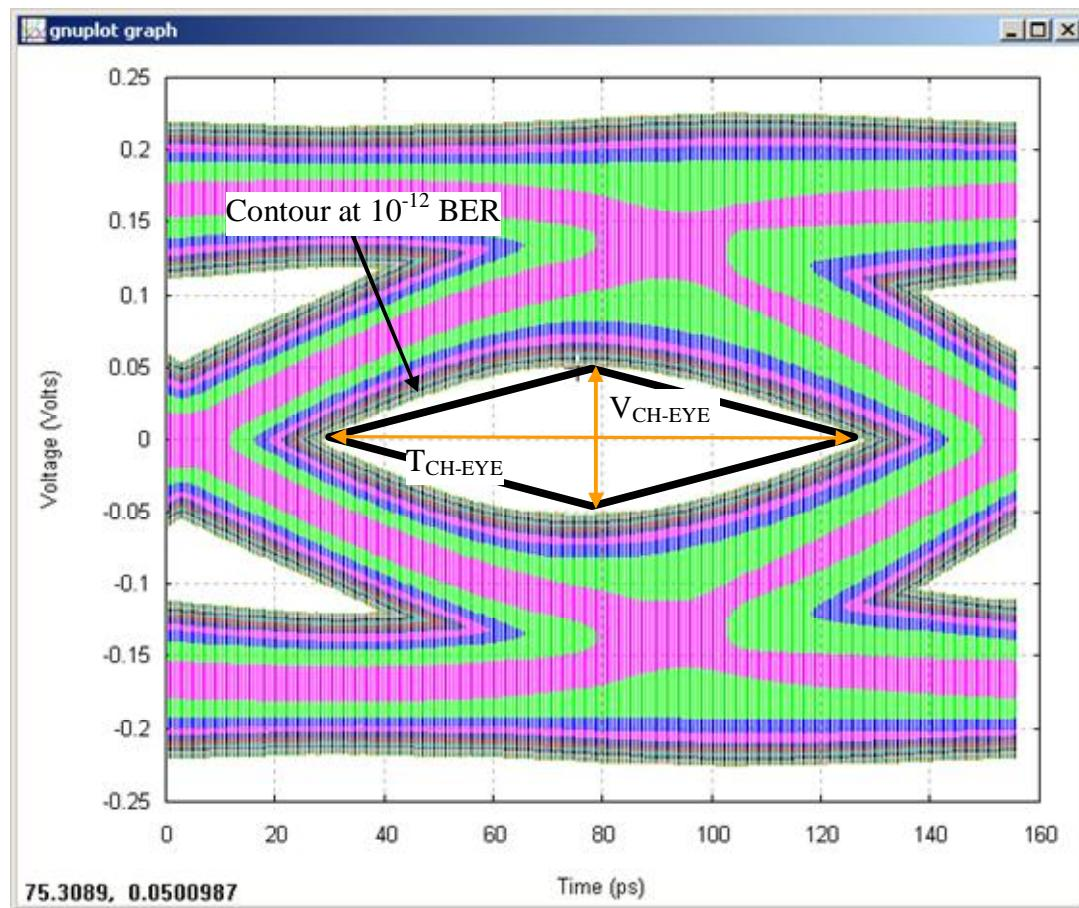
**Figure 57. Channel compliance eye diagram**
